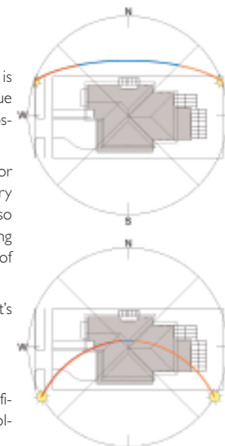
Top Winter solstice sun path for Sydney identifying the proportion of sun in each segment of the sky. The majority of the sun is in the northern segment. Eastern and western facades have very little solar exposure at this time.
